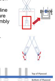
Step 39. Place the cross back in position with the leaves of the hinges over the bolts. Place washers and nuts on the bolts and tighten.
